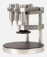
Watch holder allowing a perpendicular 5N strain on crown and / or on pushers.
